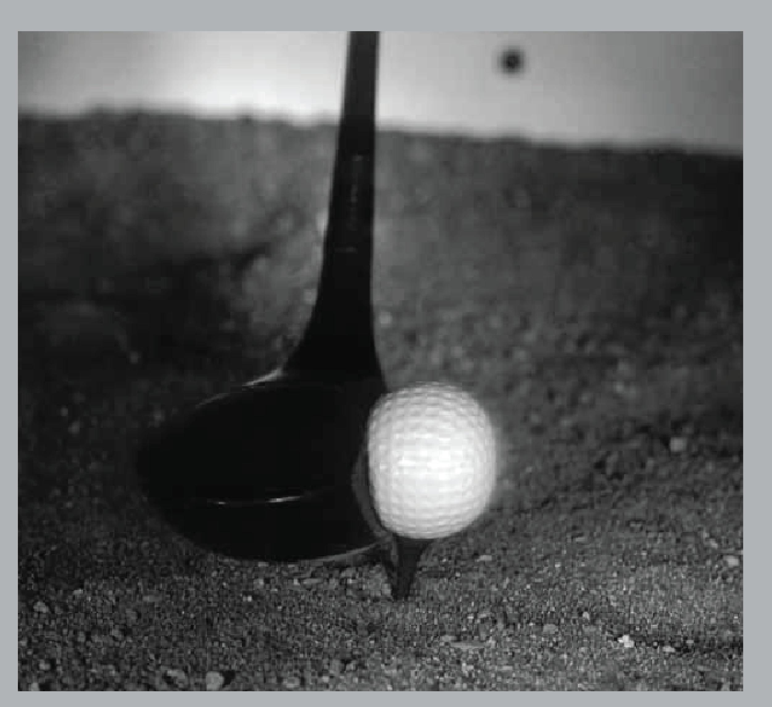
This 1935 photograph shows that even a light stroke will compress a golf ball. The exposure is 1/50,000th of a second.
