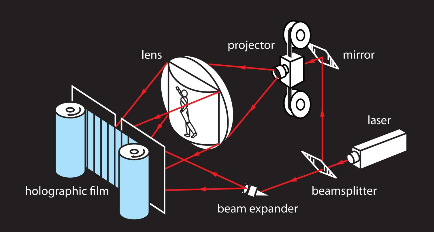
Each movie frame is made into a thin, vertical hologram. These holograms all go on the same piece of film.
