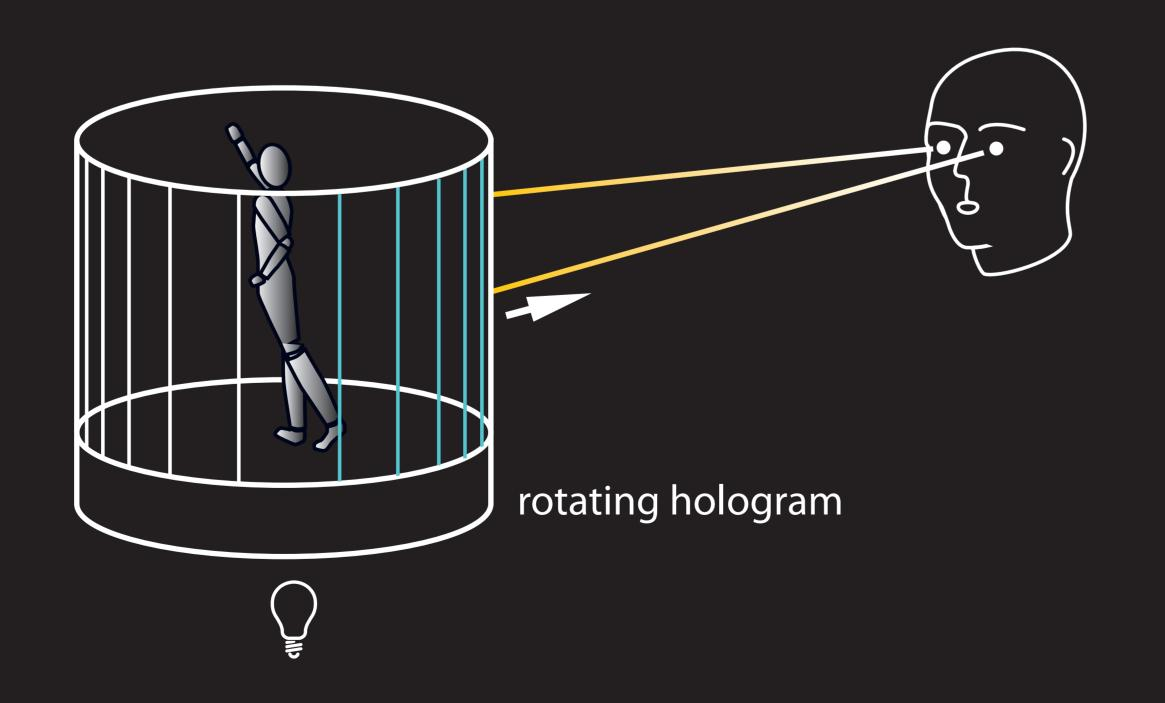
The holographic film is flipped and lit with a divergent light source. Each eye sees a different hologram, a stereo pair of images that results in a 3-dimensional illustration. As the cylinder turns, the eyes see different pairs of images, producing a moving image.
